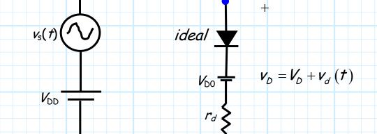
If the DC voltage source is sufficiently large (e.g.,  $V_{DD} \gg V_{D0}$ ), we will find that the ideal diode is forward biased ( $v_D^i = 0$ ):
